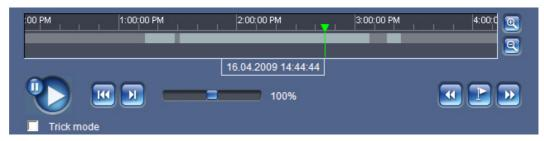
You will see a time bar below the video image for quick orientation. A green arrow above the bar indicates the position of the image currently being played back within the sequence.
